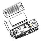
3. Ensure that the gap in your SIM card and the gap for the SIM card slot point in the same direction and that the side with a metal part faces down. Then slide the SIM card into the SIM card slot.
