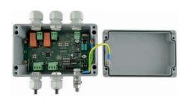
A 230VAC/24/36/48VDC power pack is installed upstream from the 4-channel control unit. The power pack is equipped with integrated protection against overloading and short-circuiting, with automatic or manual reset.
