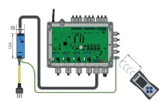
The cold conductor monitoring is used for detecting defective installations or lights that are not connected. The monitoring is automatically activated as soon as the lights are switched off.
