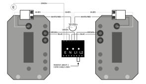
Typical wiring diagram - emergency luminaires
