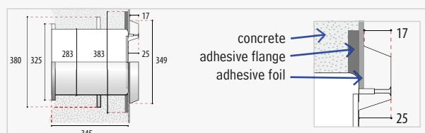
[60] later installation (tiles + mortar 15–20 mm)
