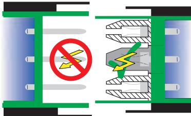
eXLink is a complete system for connecting and disconnecting product electrically. This system is available in different versions for different applications: 4-pole, 4-pole + PE and 6-pole + PE.
