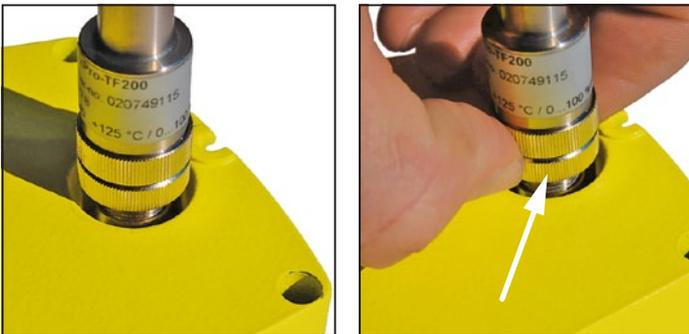
For mounting the sensor must be plugged into the socket and screwed on the sensor by turning the lower knurled screw clockwise. Tighten hand-screwed only. A small clearance between transmitter and sensor has to be accepted due to production conditions.
