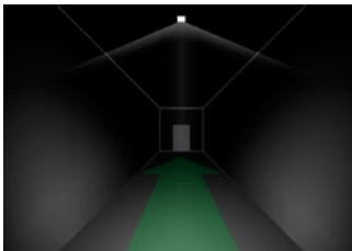
Escape route illumination with symmetric optics
