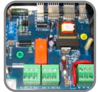
DC POWER SUPPLY
