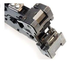
Insert the system cable into the metal bracket and turn it until it lies flat in the bracket. The negative pole (white marking) must be aligned toward the front of the pliers and correspond with the + and - imprints on the sides of the pliers. Operate the crimping pliers.
