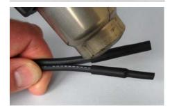
Compress shrink tube ends in the hot condition
