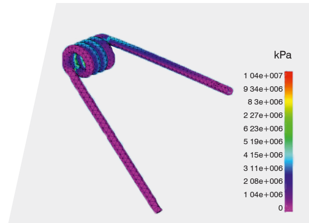
Newson Gale springs are designed and analysed with the aid of Finite Element Analysis technologies.
