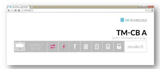
After successful configuration of the network connection and entering the set/received IP address in the web browser, a website should be displayed. The website allows to quickly preview the system status.
