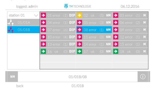
After logging in, the user can change the configuration of the fitting operation. It is necessary to select the frame and in the menu we have to choose the change of the work mode and change the description, in addition, the name of the binding is printed in the middle. After changing the operating mode, the record icon is activated on the right.
