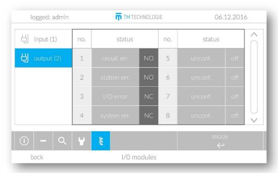
Output module is used to indicate the system status. Module outputs are opened and closed with a relay. The user configures each output by setting response to one of the five possible errors in the system:
