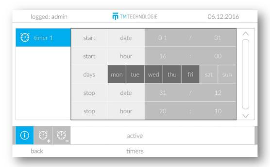
The system allows to add 64 independent timers. Timers are used to control the night groups. The following parameters can be set in each timer:
