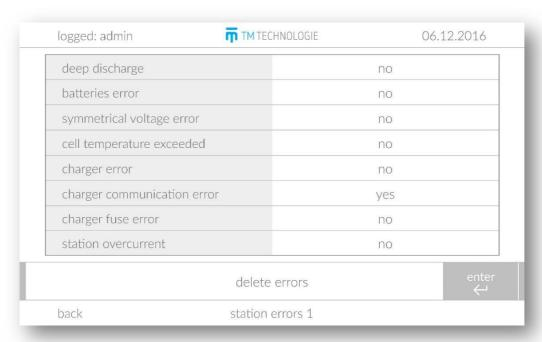
List of errors detected in the substation. Once the fault is remedied, the user must manually reset errors.
