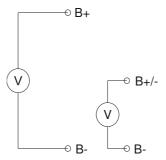
Voltage measured on the circuit (B+), (B-) should be positive. It should be 220 V +/- 30 V and approximately 2 times the voltage measured on the circuit (B+/-), (B-).
