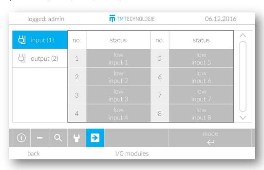
Input module is a module used to control the system elements. It consists of eight inputs (control by closing or supplying voltage – depending on the model). In the input module window, the user can check the current status and description of all inputs.
