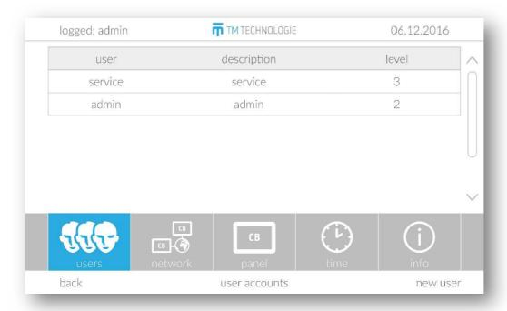
The menu contains a list of users added to the system. The system allows to add 250 users. The item on the list consists of the following elements:
