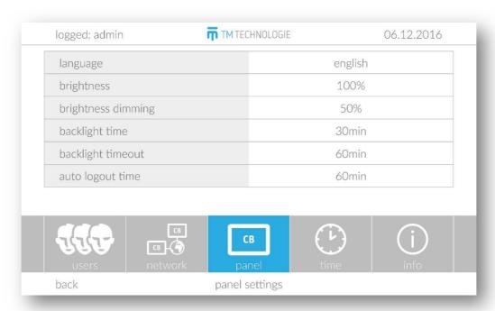
The tab is used to configure the panel settings. The user has the ability to change:
