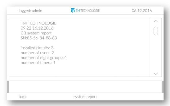
Reports are documents describing the system status and presenting the results of fitting tests in the system. Reports are generated monthly (at midnight of a new month) or on user request. Reports can be copied to a portable data carrier after its connection. Each report includes:
