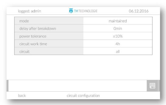
The window allows to change the operating parameters of the circuit:
