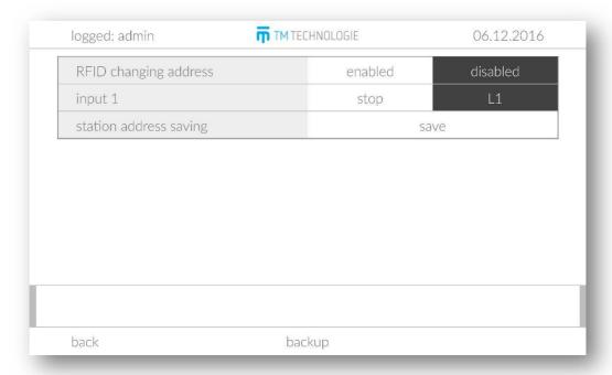
The tab allows to lock and prevent the fitting addresses from being changed through wireless programming. Once the option is changed, the systems sends a command to all fittings. Saving station address applies addresses set on the DIP switches. The user can choose whether the L1 input is to serve as a phase monitor or so-called Total Stop. If selected:
