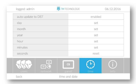
This window allows to correct the date and time. After being switched on by the user, the panel should display the correct date and time. If there was a clock desynchronisation, then the user must set the current time.
