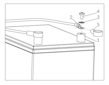
On the wires (2), slide the covers (5) (in the set). Connect the wires (2) to the battery connectors (1) using washers (3) and screws (4) (in the set). Tighten the bolts with torque: for M5 - 3 Nm, and for M6 - 5.2 Nm. After tightening the screws (4), put covers (5).
