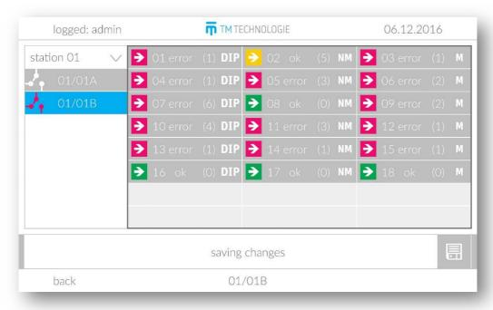
After selecting fitting details, the system displays a list of fittings monitored from the circuit.
