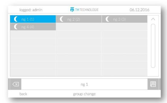
In the circuit details window, after selecting the group change option, the system displays a list of available groups. To change the group, select another group and confirm the change by pressing . To remove the circuit from the group, press the cross icon on the toolbar and confirm.
