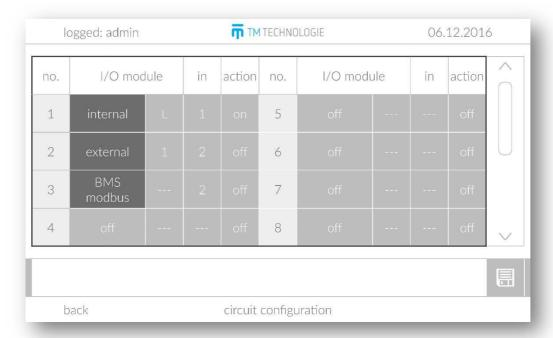
The window allows to configure the operating status of the circuit to respond to external triggering. The user can control the circuit via the internal phase loss detecting module or the external I/O module.
