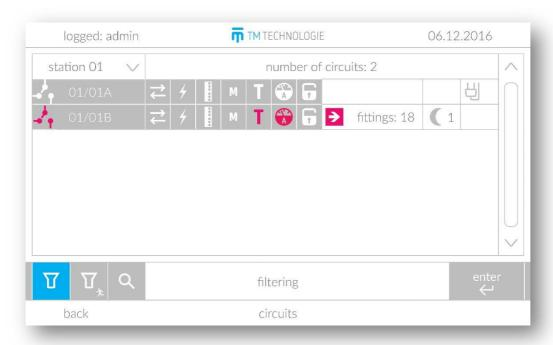
The circuit window allows to preview the state of circuits installed in the system. Click on the station/group to collapse/expand the list. Click on the circuit on the list to display detailed information.
