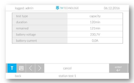
If the station is currently tested, the window is changed to display parameters of the current test. The system displays information such as test type, its duration, the remaining time, as well as battery voltage and current.
