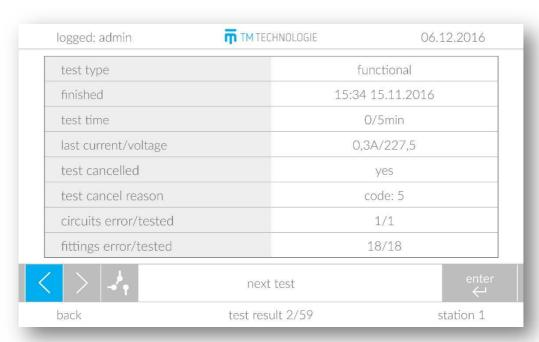
The user can browse the history of tests performed for the station. Tests are displayed from the latest to the oldest.
