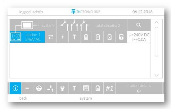
The "system" menu allows to quickly determine the system status. The first line shows information about the current state of the system, number and status of all circuits – and subsequent lines – a list of stations added to the system.
