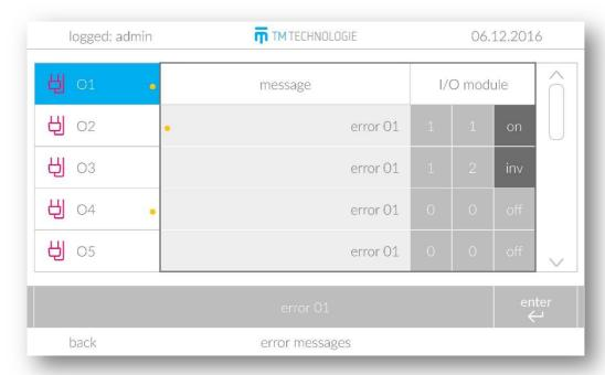
The control unit allows to display error messages in the main window of the system. It is possible to configure up to 64 error messages. The user can change the message text (up to 20 characters).
