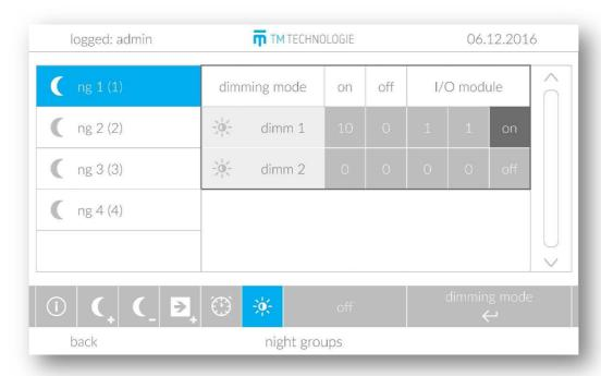
Dimming mode is the operating mode of the night group which allows the fitting to operate with a preset dimming. In response to a change of the I/O module input state, the fitting enters operation mode according to the configured, so-called group truth table.
