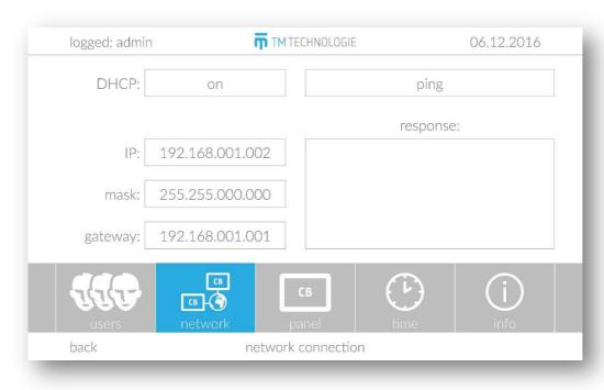
The "network" tab is used to configure the Internet connection between the panel and the user's PC. The user can connect the unit directly to a PC or to a local network in the building. If connection to a PC is preferred, disable DHCP and configure the Internet connection by filling in the fields IP, mask, and gateway. If connection to a network automatically assigning an IP address is preferred, mark DHCP as "enabled".
