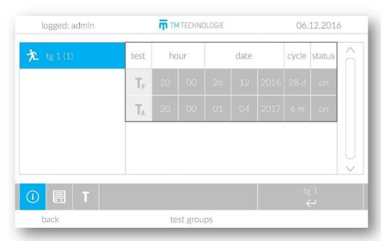
Each substation is automatically assigned to its test group. The group task is the automatic (cyclic) triggering of tests according to a preset schedule. After the test, it is automatically postponed to a new date corresponding to a preset cycle. The function test cycle can be set in the range from 1 to 28 days – and the autonomy test cycle – from 1 to 12 months.
