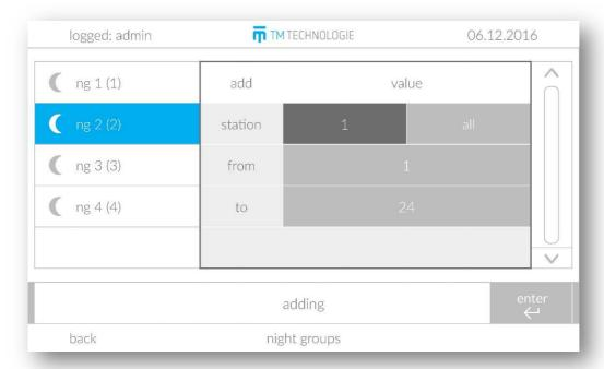
Night groups allow to add multiple circuits to one group at the same time. For this purpose, the user must select the desired group and then, on the toolbar, select the option of adding circuits to the group and confirm by pressing "enter". The system takes the user to a window where it is possible to select:
