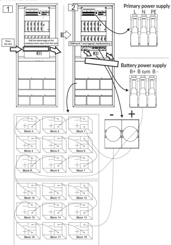
Keep the accumulator fuses removed until the final commissioning!
