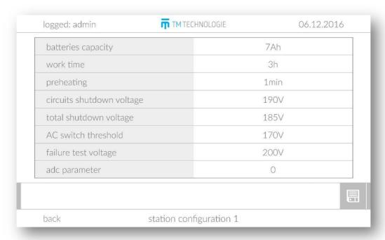
The tab is visible only when logged in. Changes in this tab can be made only by user "admin" (only battery capacity, work time and preheating) or an authorised service centre of TM Technologie.
