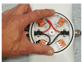
Check that there is a small O-ring in the centre of the MarkLED. (missing O-rings must be replaced without fail). Strip the conductors of the MarkLED and connect to the Wago connection terminals.
