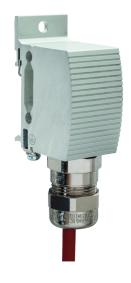
Ex-protected thermostat of temperature class T6 (max. 85 °C). High switching capacity for direct control of connected heaters. Application: Enclosures and control cabinets in explosive environments. Mechanical thermostat with high response accuracy and response speed.
