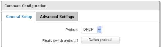
You can switch between the Static, DHCP or PPPoE protocol by selecting the protocol that you want to use and then pressing **Switch Protocol**.
