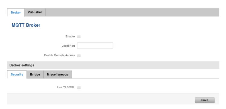
In order to use TLS/SSL for connecting clients (subscribers and publishers) to the broker, the one should check *Use TLS/SSL*. After that, additional settings will be displayed to the user as shown below. Here the user can upload certificates, key files and choose TLS version, which will be used for data encryption between broker and clients (subscribers and publishers)
