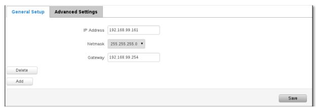
As you can see, the configuration is very similar to the static protocol; only in the example a 99th subnet is defined. Now if some device has an IP in the 99 subnet (192.168.99.xxx) and the subnets gateway metric is "higher" and the device is trying to reach the internet it will reroute it's traffic not to the gateway that is defined in common configurations but through the one that is specified in IP aliases.
