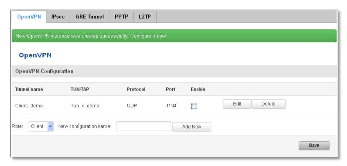
To see at specific configuration settings press "edit" button located in newly created configuration entry. A new page with detailed configuration appears, as shown in the picture below (TLS client example).
