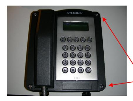
Put upper part of telephone onto lower part of housing and fasten with 4 cover screws (torque 3Nm, wrench TX30)
