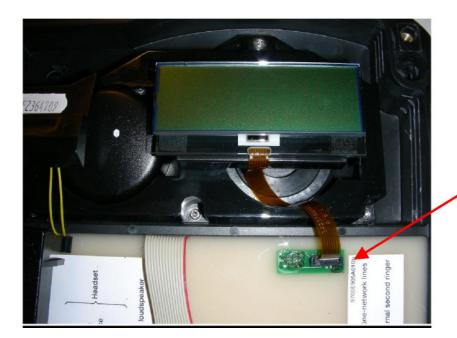
Place the new display in the centre of the mounting frame. Attach connecting line to zero insertion force connector and lock.
