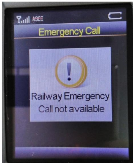
**Note:** If the above information is displayed on the screen, it indicates that the SIM card is not authorized for the railway emergency call. In this case, please hand over the faulty SIM card to relevant GSM-R department, and use a functioning SIM card instead.
