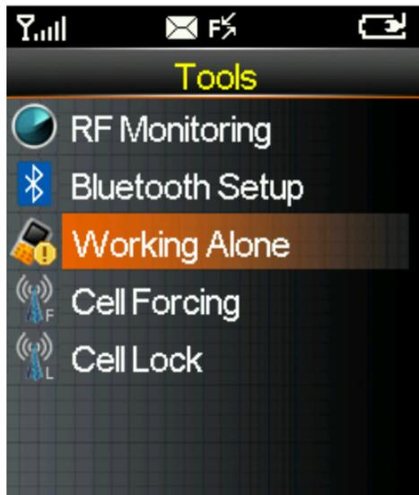
**"No Motion Alarm"** mode : The handset remains stationary without any operation on it in a preset time;
