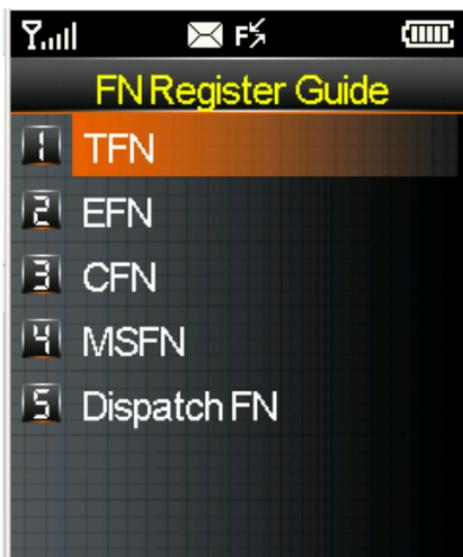
Choose **TFN** to display the function number registration page. After you enter relevant information, press the **OK** key. In the case of the train shunting mode, enter five-digit train number (pad zeros if the train number has less than five digits).
