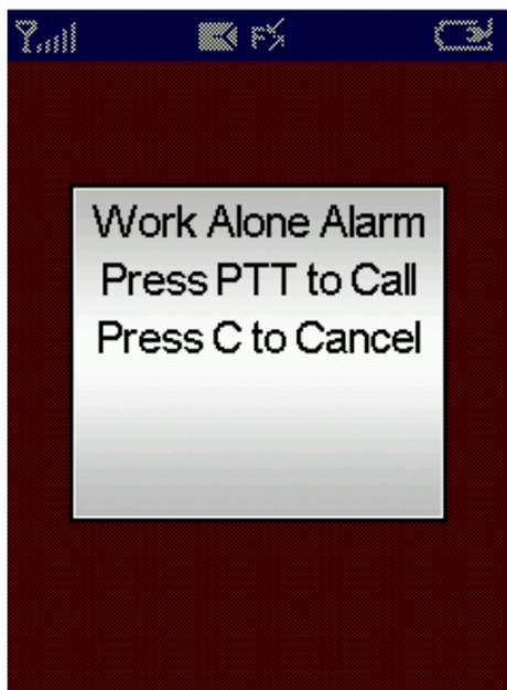
Similar to manually initiating Working Alone emergency alarm, the OPS can automatically initiate a alarm call from the terminal device to the receiving station. In addition, an SMS message including the OPS location data is also sent to the receiving station. The staff of the receiving station can know the current location of the terminal device from the screen, and take corresponding measures.
