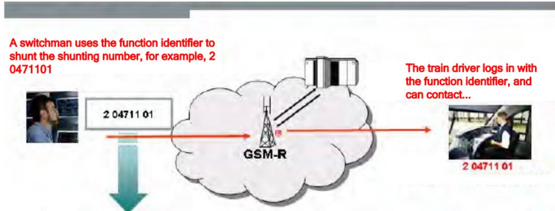
**Note:** The driver needs to use correct function identifier matching the shunting number to log in. Therefore, you can use Leading Driver function number to find the driver.
