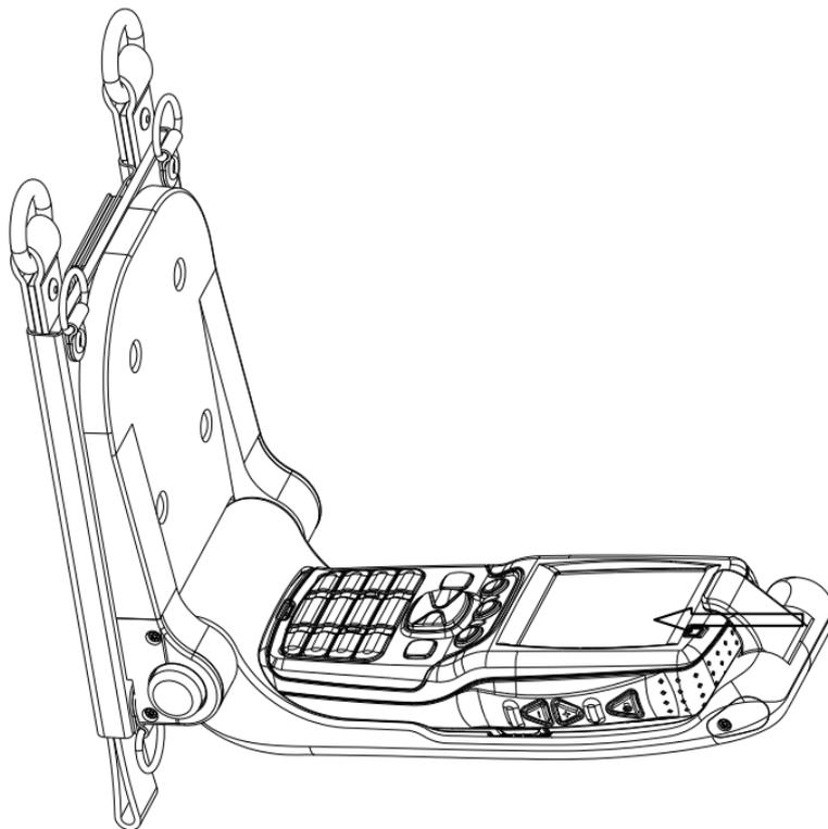
After the clamshell is open, insert the OPS from top to bottom into the holder. Press & hold the locking apparatus until the device is engaged in.
