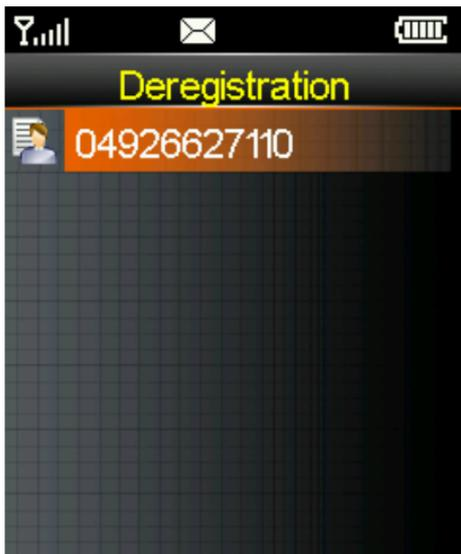
Press the **OK** key to display the main menu, choose **Identity>Deregistration** to display the deregister the function number UI, and press the **OK** key.
