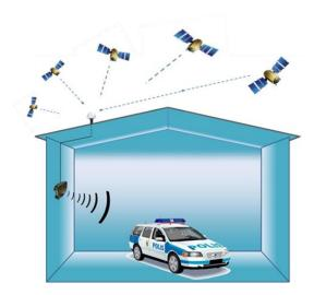
To use GNSS satellite devices inside your building you will need a repeater system to transfer the outdoor signals to inside. A repeater is a device that relays GNSS signals to any indoor location that isn't normally reachable. The repeater receives GNSS satellite signals via an antenna located outside the building and reradiates them to the indoor or covered space.
